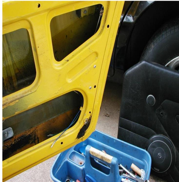
Only two holes are drilled into the door as pictured to position the lock actuator motor parallel with the door lock rod that goes to the top of the door. You can see the connector that attaches the two rods together. The door lock actuator wires are run in the same holding tabs as the window motor.
